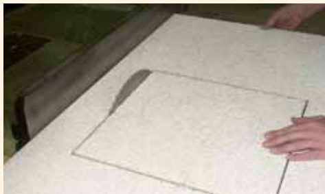
Cutting out of the opening/cover plate from the back of the panel.
