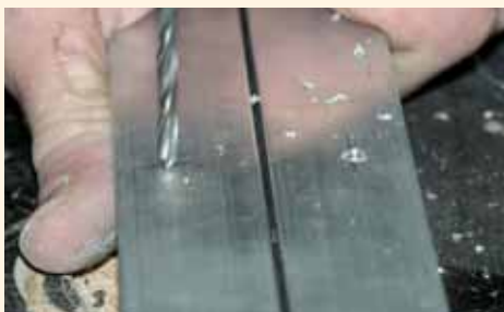
Drilling of the frame.
