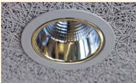
Spotlights up to diameter = 150 mm from panel thickness 15 mm, max. weight \leq 0,60 kg Downlights up to diameter = 200 mm from panel thickness 25 mm, max. weight \leq 1,50 kg Downlights up to diameter = 300 mm from panel thickness 35 mm, max. weight \leq 2,50 kg
